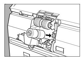
7 Set the feed rollers in place (①), and align the notch in the roller's axle with the shaft on the scanner (②).
