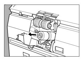
6 Place the new feed rollers on the pin.
