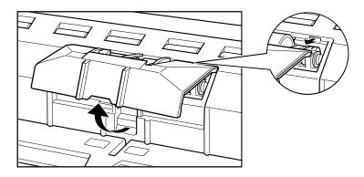
$\boldsymbol{3}$  Lift the roller clamp lever (1) and slide it to the left (2).
