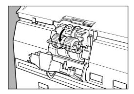
4 Position the square axle of the pickup roller on the left and insert the new pickup rollers.
