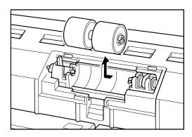
5 Set the new retard rollers in place, and align the notch in the roller's axle with the shaft on the scanner.
