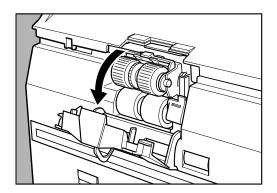
3 Open the roller holder and remove the pickup rollers.
