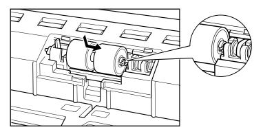
6 Slide the roller clamp lever to the right, and push it into the hole in the retard rollers.
